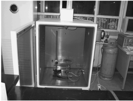
Fig. 1. Toxicity analysis apparatus of fire gases.
